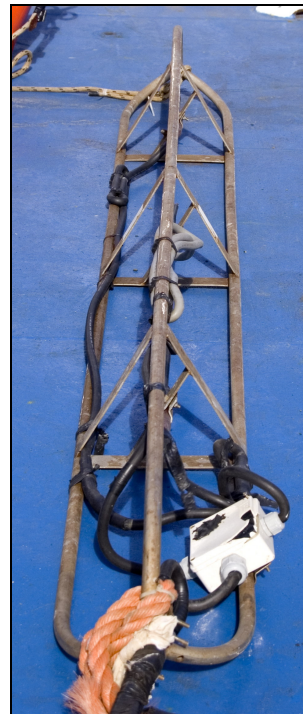
Fig. 9 Sparker source, Eg&G, 1 kJ
