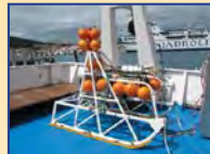
UWTV system - towed sledge, camera and multiparameter probe
