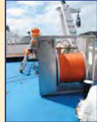
UWTV system - towing data cable and winch
