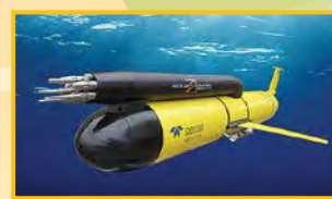
Slocum G2 glider with the Microrider installed on the top
