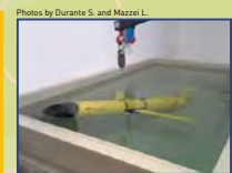
"Teresa" during ballasting procedure in the CNR La Spezia Laboratory, Italy
